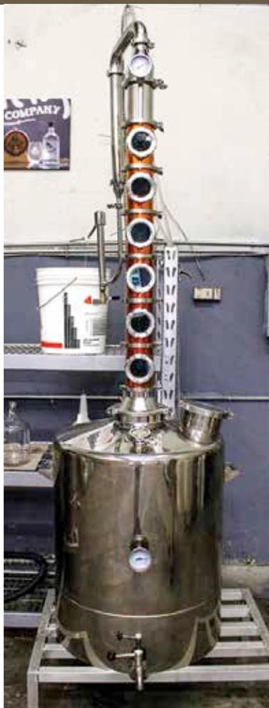
The reflux still, a tall copper and stainless steel monstrosity condenses fermented molasses into Raleigh Rum.
