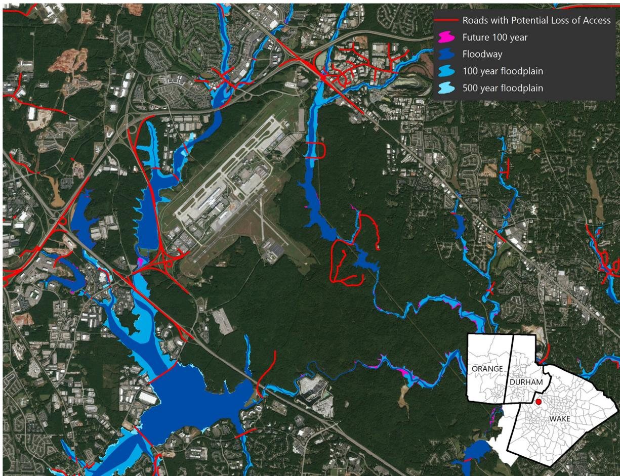
Aerial image of the Raleigh-Durham International Airport shown with roads and floodway and floodplain levels for the surrounding area. Red lines indicate roads that are either inundated or potentially cut-off or isolated. (Figure source: UNC Asheville's NEMAC. Data sources: NC Floodplain Mapping Program 2017, Open Street Map.)
