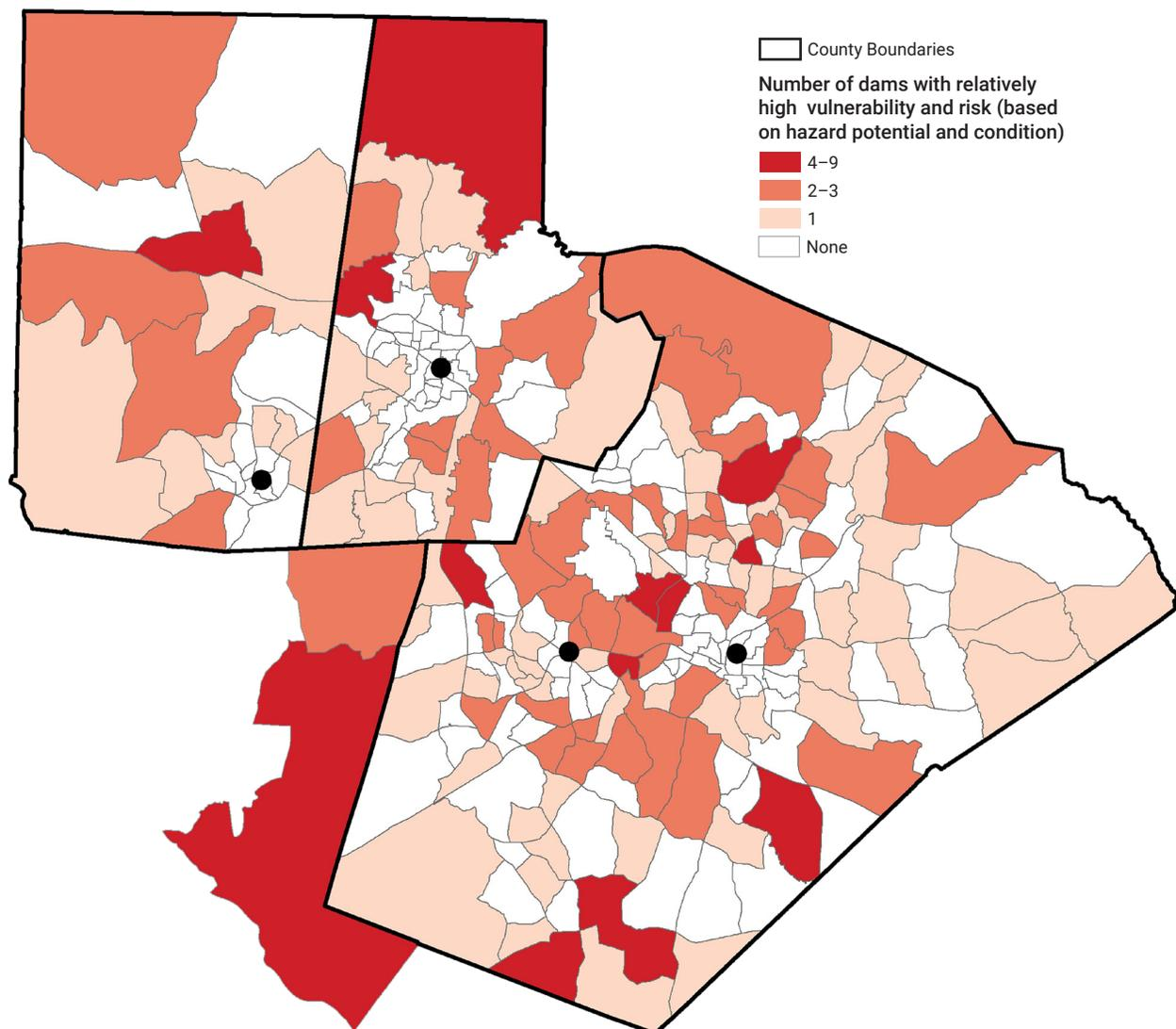
Two components were used to consider vulnerability and risk to North Carolina-regulated dams: the condition assessment and the hazard potential. The condition assessment evaluates dams with classifications of “poor,” “fair,” “satisfactory,” and “unknown.” Dams with a condition assessment of “poor” were considered to be the most vulnerable to flooding. Hazard potential is classified
