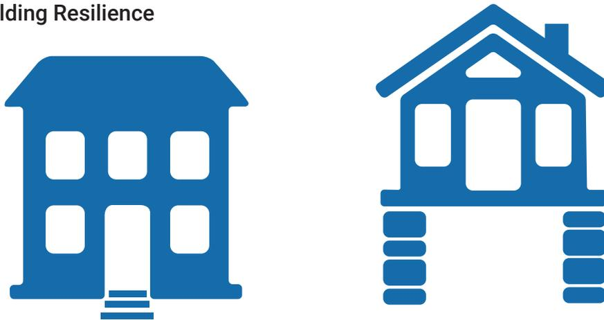
*Resilience focuses on reducing vulnerability and risk. As an example, elevating a structure can build resilience to flood inundation. (Figure source: UNC Asheville’s NEMAC.)*
