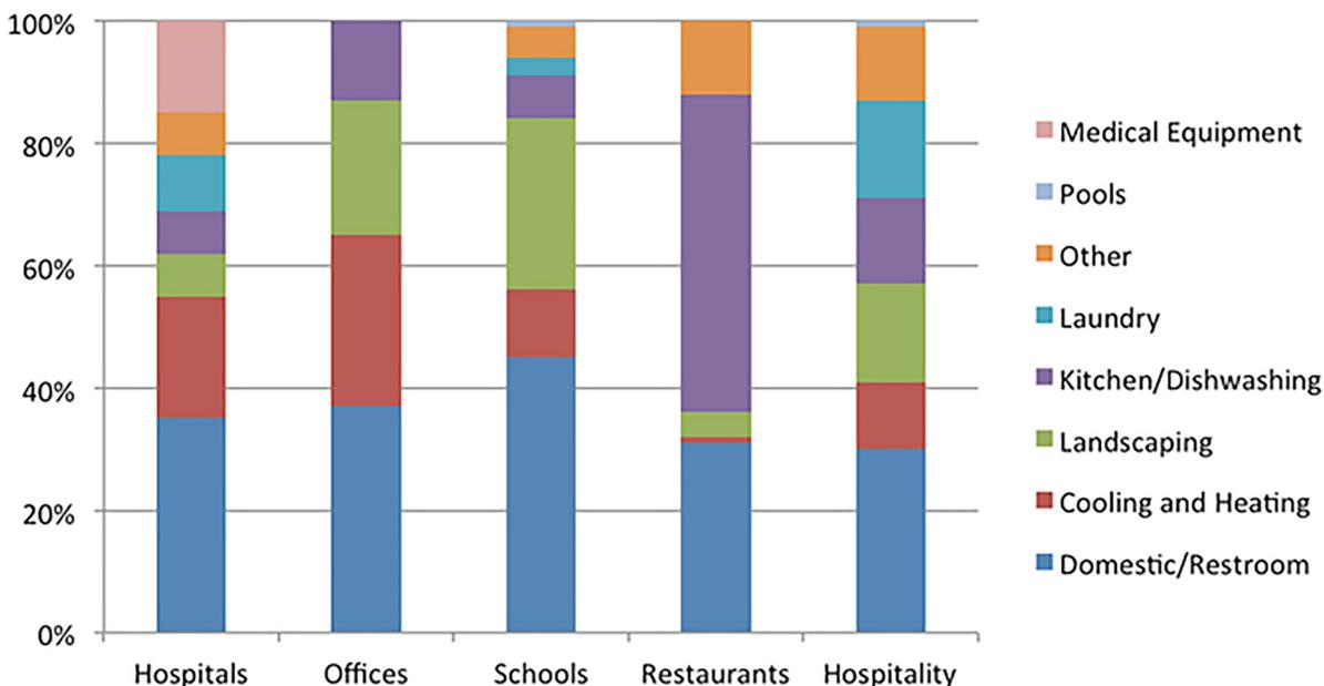
End uses of water in various types of commercial and institutional facilities. (Figure source: U.S. Environmental Protection Agency, "WaterSense: Commercial Buildings: Types of Facilities.")
