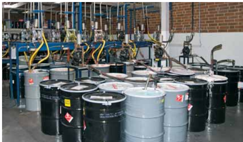
Computerized technology drives the manufacturing operations. Ink is fed directly from barrels to the presses, with color mixtures determined by computers.
