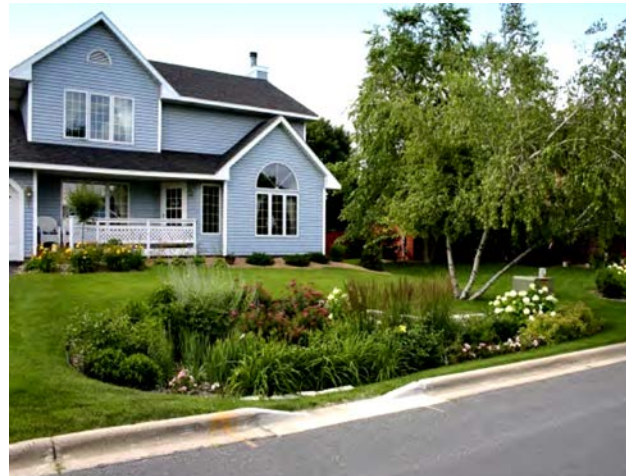
Figure 7-3. A house with a rain garden utilizing native landscaping. Notice the curb cut that allows street runoff to reach the rain garden.
