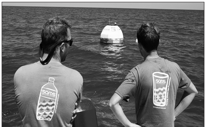
PHOTO COURTESY OF SAROS Chris Matthews (left) and Justin Sonnett, co-founders of SAROS, watch their invention, a wave-powered buoy that desalinates water and makes it clean to drink, float on the water.
